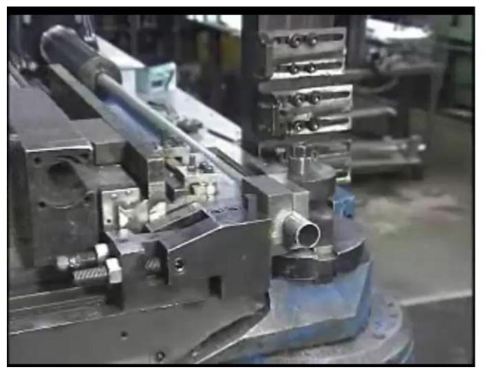
Reduces crushing of inner bend radius
