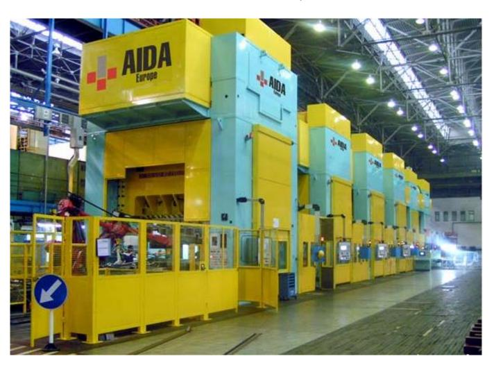
**Transfer Press** – sheet fed, single press action with multiple dies attached to platen and transfer mechanism
