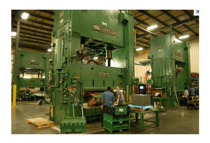
**Stage Tooling** – manual presses organized in a production line with manual transfer of parts between presses (popular in low labor cost
